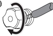
C. Tighten Cap to Secure Wire
